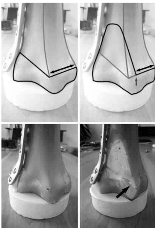
Fig. 7 View of SP ( left ) and BP ( right ) techniques, outlined in black is the shape of the distal part of the OT. Grey arrow ( top right ): the ascending saw cut endpoint on the lateral cortex. Black arrows ( top left and right ): the size of the intact lateral cortical hinge. Clearly visible ( bottom left and right ) is the difference in fracture pattern of the lateral cortex in the torsion failure test. Black arrow ( bottom right ): the lateral cortex fracture at the endpoint of the ascending saw cut
