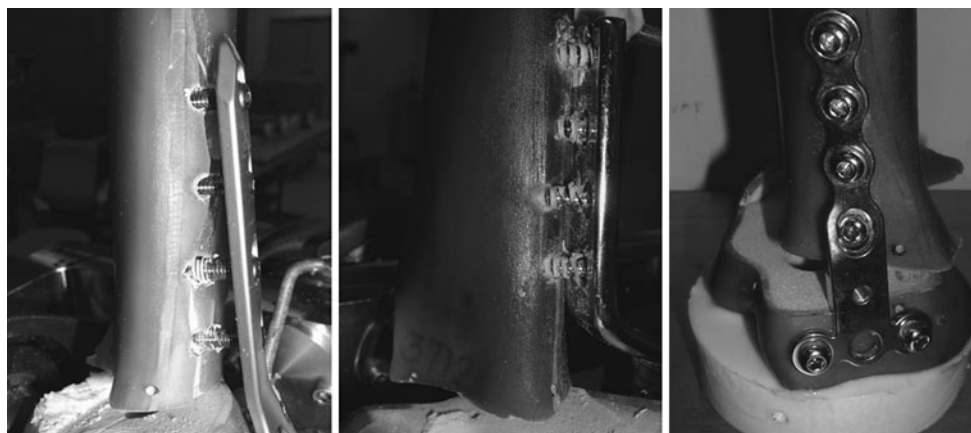
Fig. 6 Detailed view of the failure patterns in the torsional failure tests. Fracture of the femur at the screw–bone interface in the MDF in the torsional failure tests ( left ).The screws have clearly been bent at
